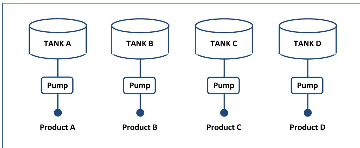
Tanks, including pumps and piping, represent large investments. If it was possible to install a blending unit at the distribution terminal only tanks for the base grades would be needed and for each intermediate grade distributed, one tank with piping could be saved.
