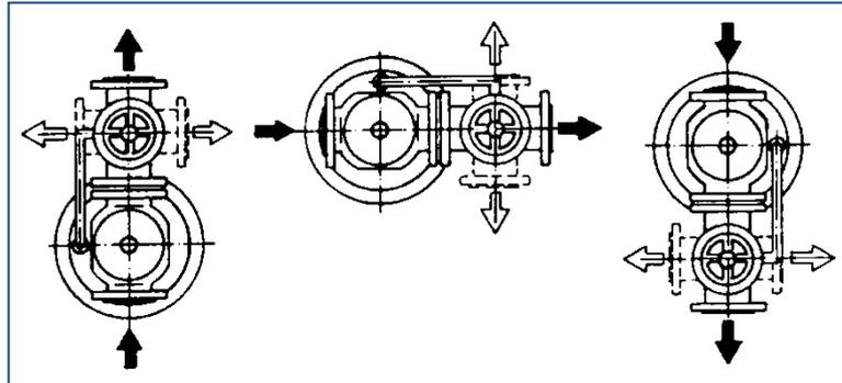
The inlets of the blending unit are equipped with check valves to stop flow from one component pipe with higher pressure to the other component pipe, when the flow in the pipe from the blending unit is shut off.
