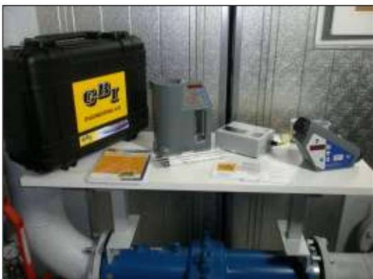
CBI / Kittiwake Fuel Oil Test Kit / Viscosity and Density
